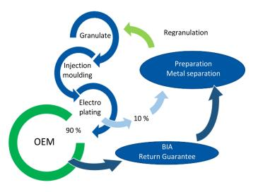
Due to the technical feasibility of separating all recyclable materials used in the manufacture of chrome-plated plastic components, these can be almost completely separated in the recycling process and then used to manufacture new products and surface finishes of similar value. As early as 2023, the FGK members guarantee that all components will be taken back completely after the product life cycle and that they will be fed into the recycling process.
